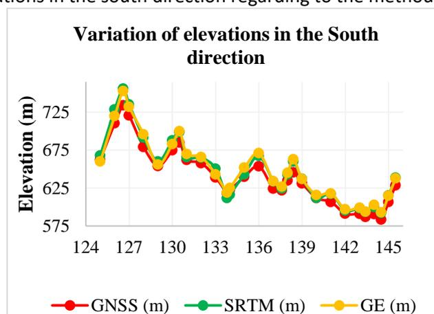
In Figures 5 and 6, it is evident that, in both the North and South directions of the surveyed section, the elevation values obtained through GE are generally higher compared to those obtained from the GNSS receiver and SRTM.
