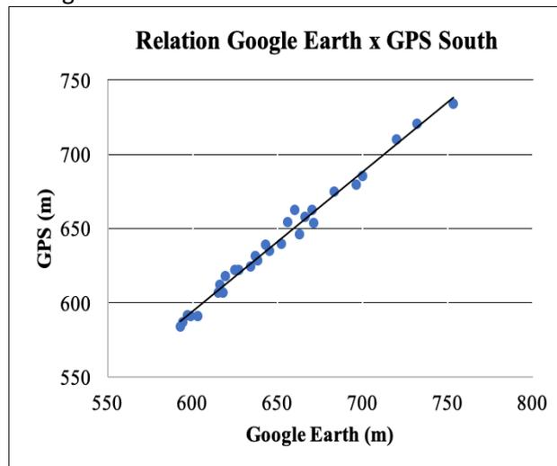
The obtained determination coefficients ( $R^2$  values) exceeding 0.98 align with findings in the literature, particularly studies that compare GNSS data directly collected with data indirectly acquired through digital terrain elevation models (ASHRAF; AHMAD; IQBAL, 2012). These results indicate a strong correlation and agreement between the methods, with minimal data dispersion. Thus, the applied approach in the road environment demonstrates its efficiency.
