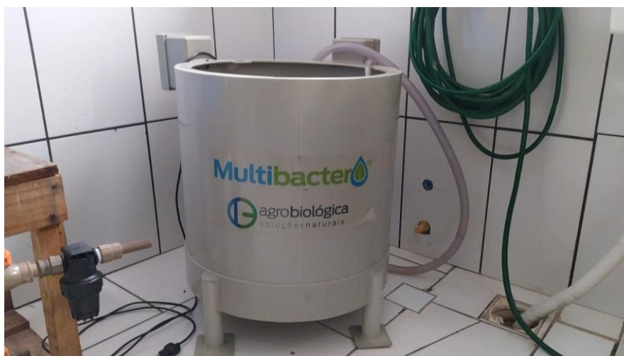
Figure 1. Venturi model bioreactor for multiplication of A. brasilense bacteria in the on farm system.
